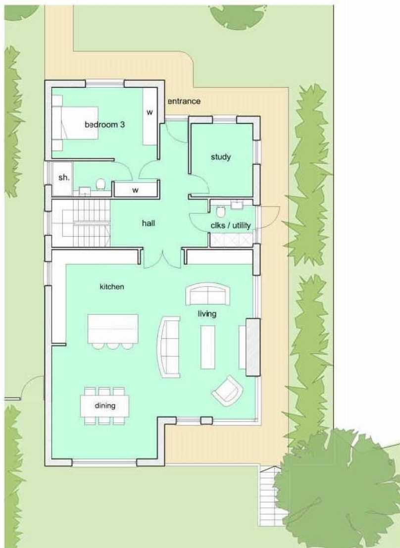
Proposed ground floor plan Scale 1:100 @A3
